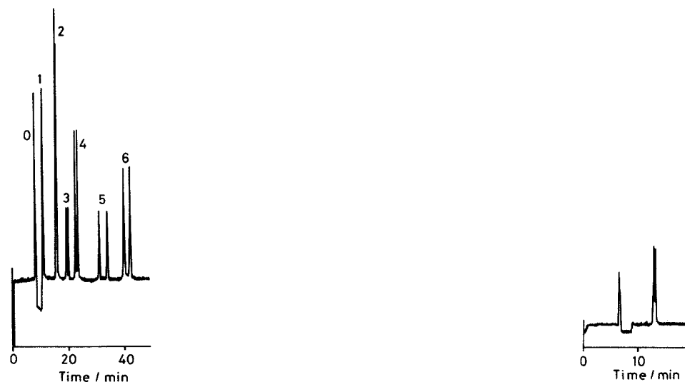
Fig. 1. Chiral separation of six PTH-DL-AA by MEKC. Corresponding amino acids: 1 = Ser; 2 = Aba; 3 = Nva; 4 = Val; 5 = Trp; 6 = Nle. 0 = acetonitrile. Micellar solution, 50 mM SDVal–30 mM SDS–0.5 M urea (pH 9.0) containing 10% (v/v) methanol; separation column, 650 mm \times 0.05 mm I.D.; length of the tube used for separation, 500 mm; total applied voltage, 20 kV; current, 17 \mu A; detection wavelength, 260 nm; temperature, ambient.
